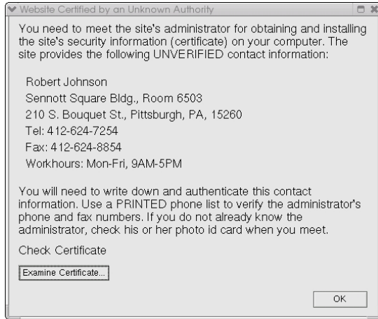
Figure 4: CSCV dialog when user is internal member of the organization that owns the accessed server.
